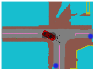
Fig. 5. Perturbation: the orientation of the car is perturbed by an angle \theta and the occupancy grid so formed detects the same set of waypoints.
