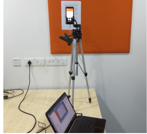
Fig. 1: The capturing set-up used for creating the proposed dataset. The document is fixed on a surface parallel to the camera plane and the focal distance is computationally varied.
