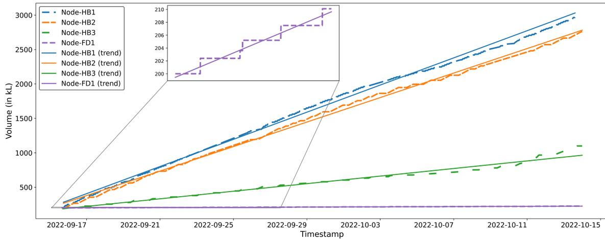
**Figure 5.4** Time series plot for net water volume in kL. The dotted thick line shows the raw data for each node from September 17, 2022 to October 15, 2022. The solid thin lines of the same color shows the best fit linear trend line corresponding to each node. (Best view in coloured)
