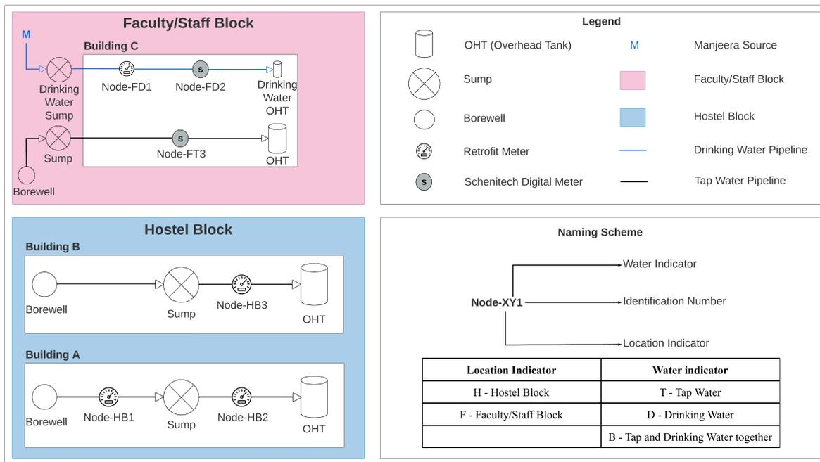
**Figure 5.1** The region in blue colour denotes Hostel Blocks, containing two student hostels, and the region shown in pink colour is for the residential block which shows water distribution for the building in the region, namely Anand Nivas
