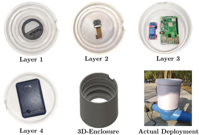
Figure 3.2 3D structure and deployed model
