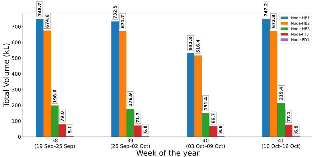
**Figure 5.6** Weekly net water supply plot over 4 weeks.
