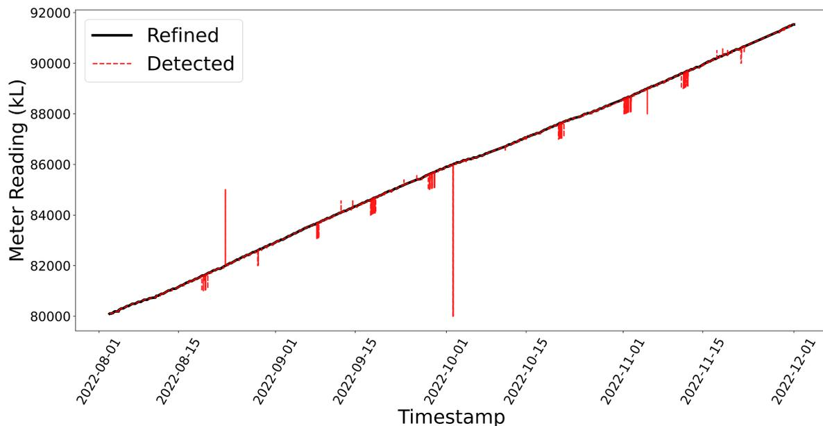
**Figure 5.3** Graph of detected values and refined values for node Node-HB2, plotted over four months of data. On the X-axis timestamp is given, and on the Y-axis, meter readings in kL (Kilo Litres) is mentioned. (Best viewed in coloured)
