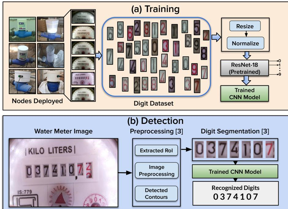
**Figure 4.2** Algorithmic pipeline for the DL methodology proposed. The dataset collected from different nodes mentioned in section 4.2 is used to train the ResNet-18 model (last layer having 10 nodes) using transfer learning mechanism. At the detection phase, preprocessing used in was used to segment the digits from water meter image. Finally the digits are recognized using the trained CNN model. (Best viewed in color)
