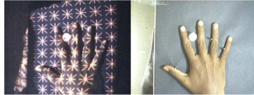
Figure 5. The hand under structured illumination as well as normal lighting. The mirror to the left enables us to compute height of palm at specific points.
