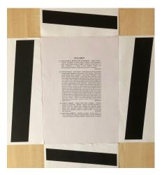
**Fig. 1**. The figure shows a typical image and the slanted edge arrangement used to create the SFR dataset. The slanted edges are placed on all sides of the document. We use four slanted edges to capture the motion and out-of-focus effects robustly. The degradations in slanted edges due to these factors lead to a low SFR score, which in turn results in a lower ground truth value for all the affected patches.
