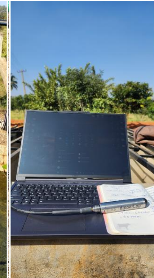
Retrieving data from water level sensor
