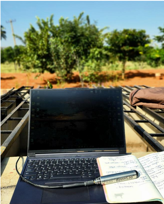
Water level sensor
