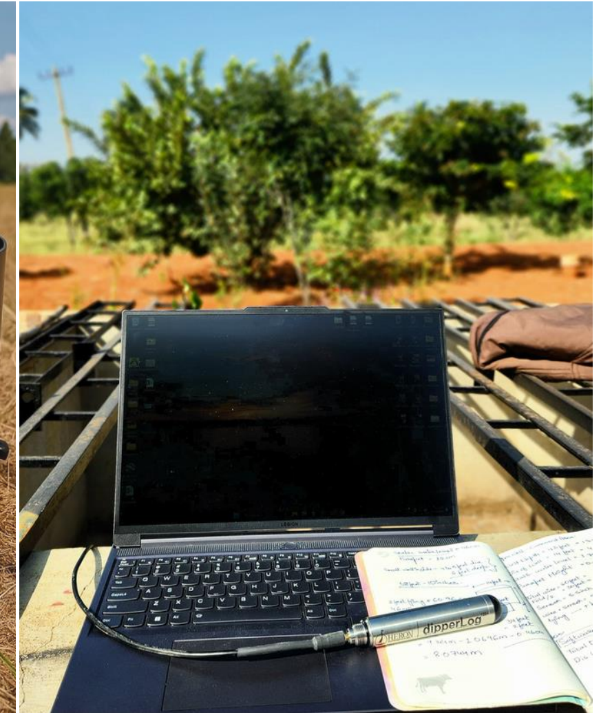
Water level sensor
