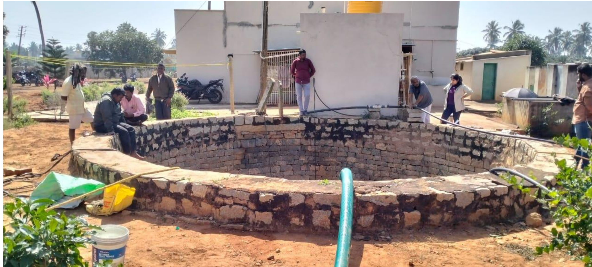
Pump test in Open wells to understand the Aquifer characteristics
